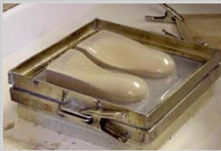
Left: Heated polypropylene vacuum-formed over wood positives
