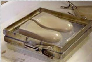
*Left: Heated polypropylene vacuum-formed over wood positives*
